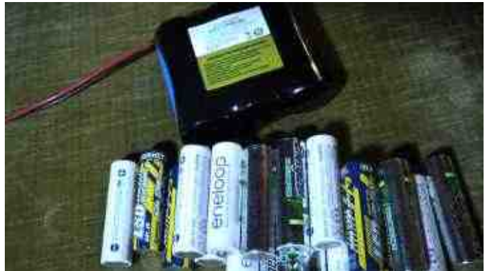
This modern lithium-iron-phosphate battery holds more power than a sizable pile of AA cells!
