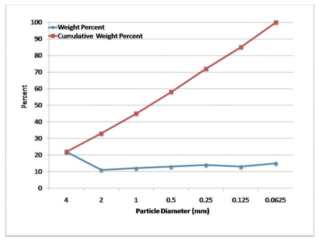
Figure 2: Cumulative Curve Particle Size Distribution
