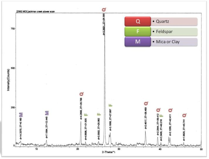
Figure 4: X-Ray Diffraction showing the concentrations of Quartz, Feldspar and Mica/Clay.
