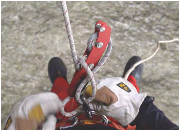
Pulling the loop through after a soft lock for a traditional hard lock-off.
