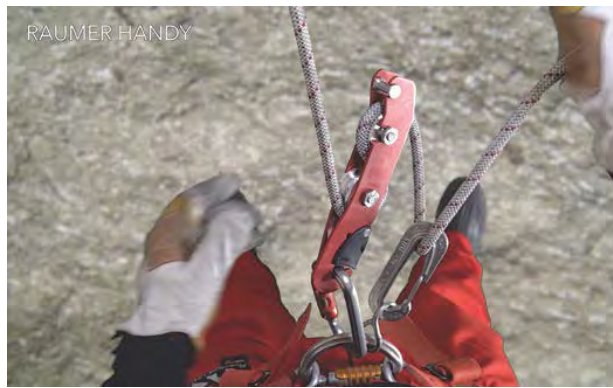
The Handy brake carabiner from Raumer with the essential “squiggle”.
