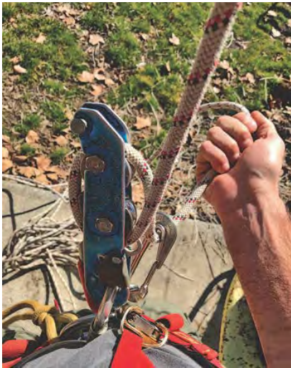
A properly done "C" rig with a Handy
