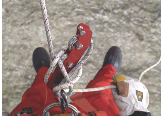
A completed, traditional hard lock-off.
